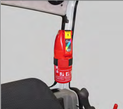
Fig. 88: Fire extinguisher on C pillar
