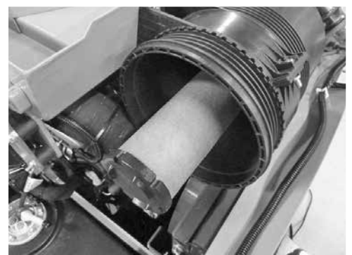
65229 Air filter, inner screen element (replace only when necessary)
