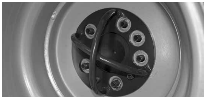
Tie down bracket on wheel hub A423091
