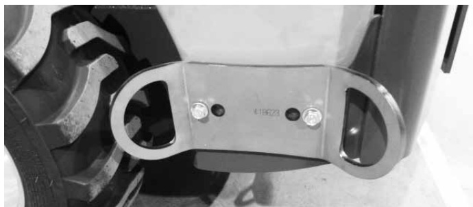
Tie down bracket A418623 installed at the side of rear frame. For side installation, two brackets are needed.
